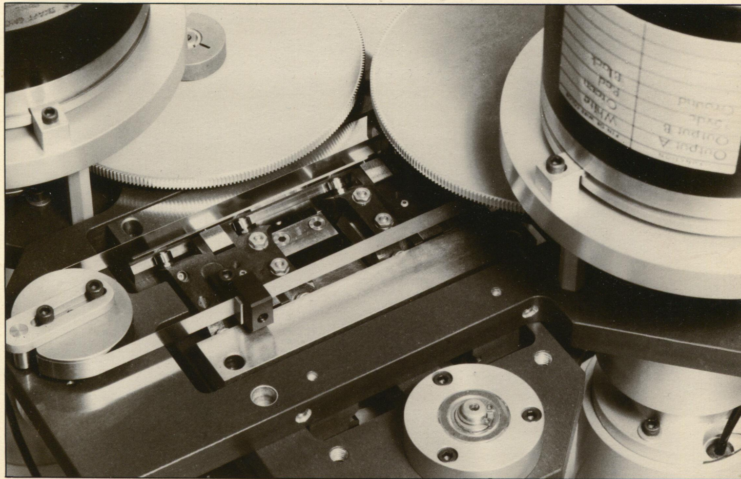
Variable Aperture Assembly* — Circuit design flexibility is guaranteed by a precision aperture assembly that can vary the size of the rectangles generated in 0.1 micron increments.
