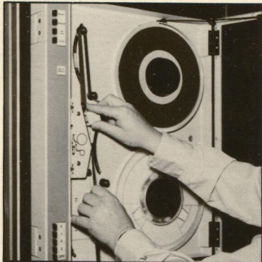
A To employ the pattern generator, the operator simply loads the magnetic tape containing digital data into the 2500 control console . . .
