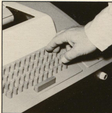
B Then he presses the "start" button, and the Combo 2500 automatically creates the desired circuit pattern on a glass reticle . . .
